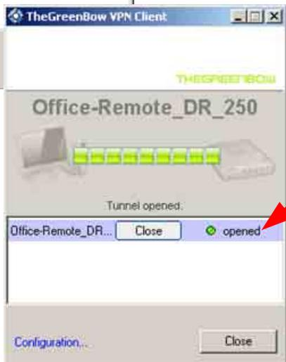
If all of the settings are correct, the tunnel will open and the status will be as shown. At this point the remote LAN is now accessible. 17
