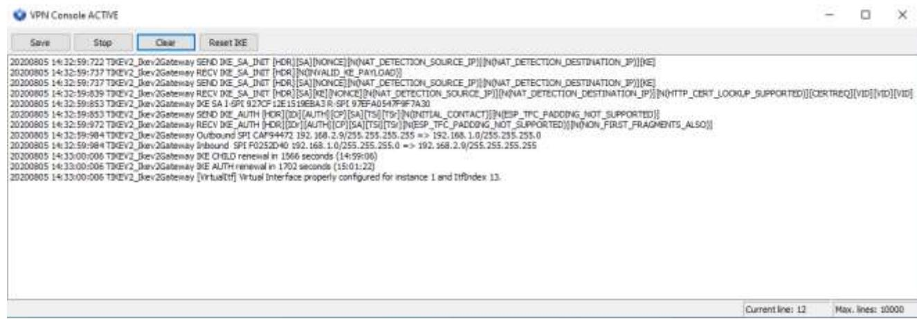
The screenshot shows the "VPN Console ACTIVE" window. At the top, there are buttons for "Save", "Stop", "Clear", and "Reset IKE". The main area displays a log of IPsec VPN events. The log entries are as follows:
