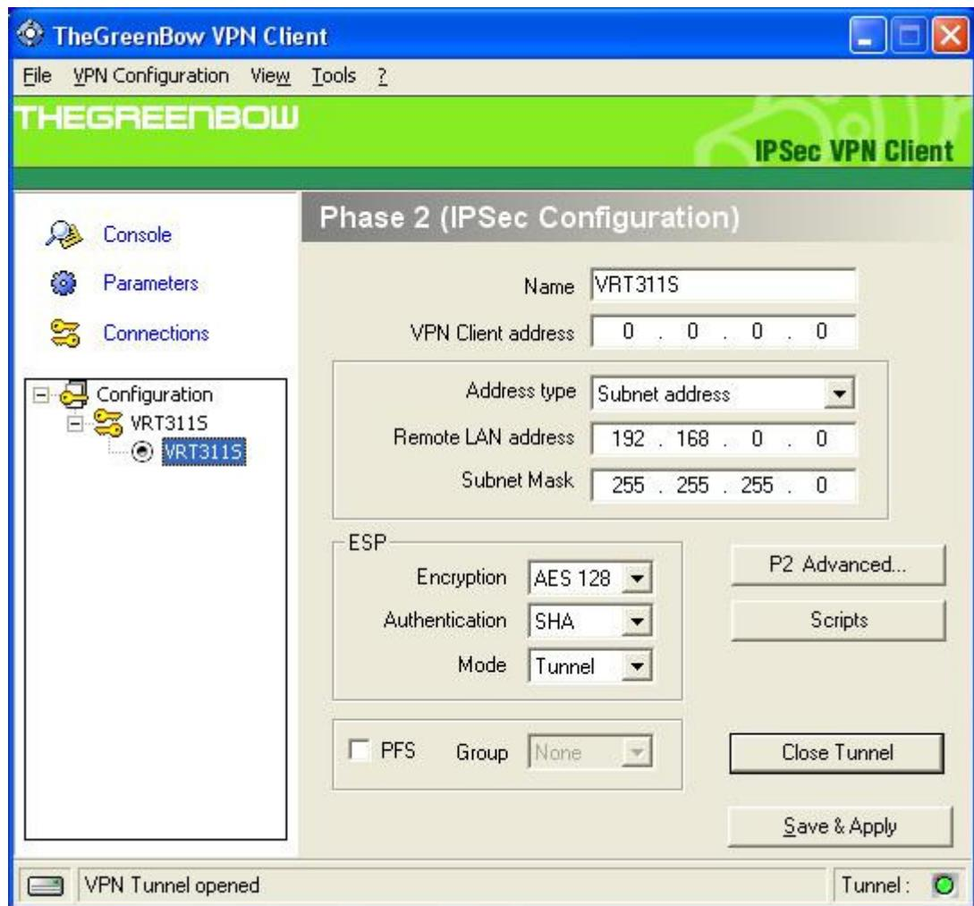
0.0.0.0 in "VPN client address" means the ip used for the vpn client is the current one on the pc's network adapter.
