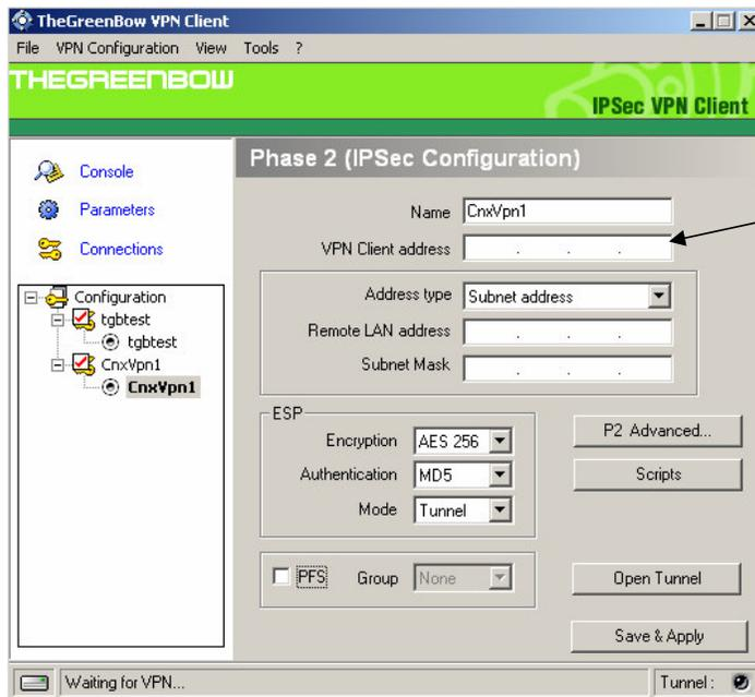
Do not define a Virtual VPN Client Address and a remote LAN network.
