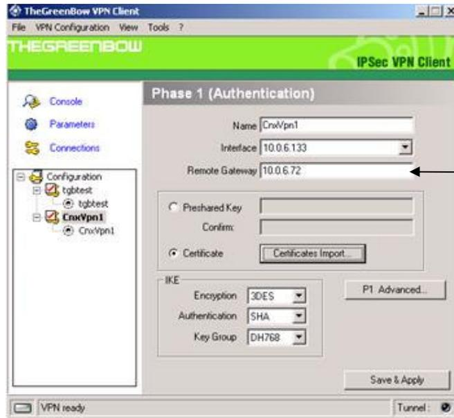
The remote VPN Gateway IP address is either an explicit IP address, or a DNS Name
