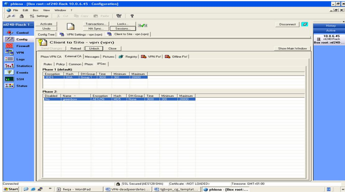
2) Enter the common section (IKE Config Mode) and define a Personal Network and a Remote LAN to which your workstation gets access to. Assuming that the IPsec VPN Client reaches the VPN gateway with IP 214.1.2.50 you have to state explicitly that this IP address is allowed to receive Network Information from the VPN gateway. To do so define an Access Control List.
