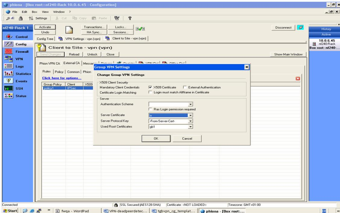
5) Create a new Rule your Policy applies to where Certificate Conditions from the IPSec VPN Client can be entered. Again the workstation IP must be entered here in order to belong to this defined group. Furthermore peer condition must be set to IPSec Client.
