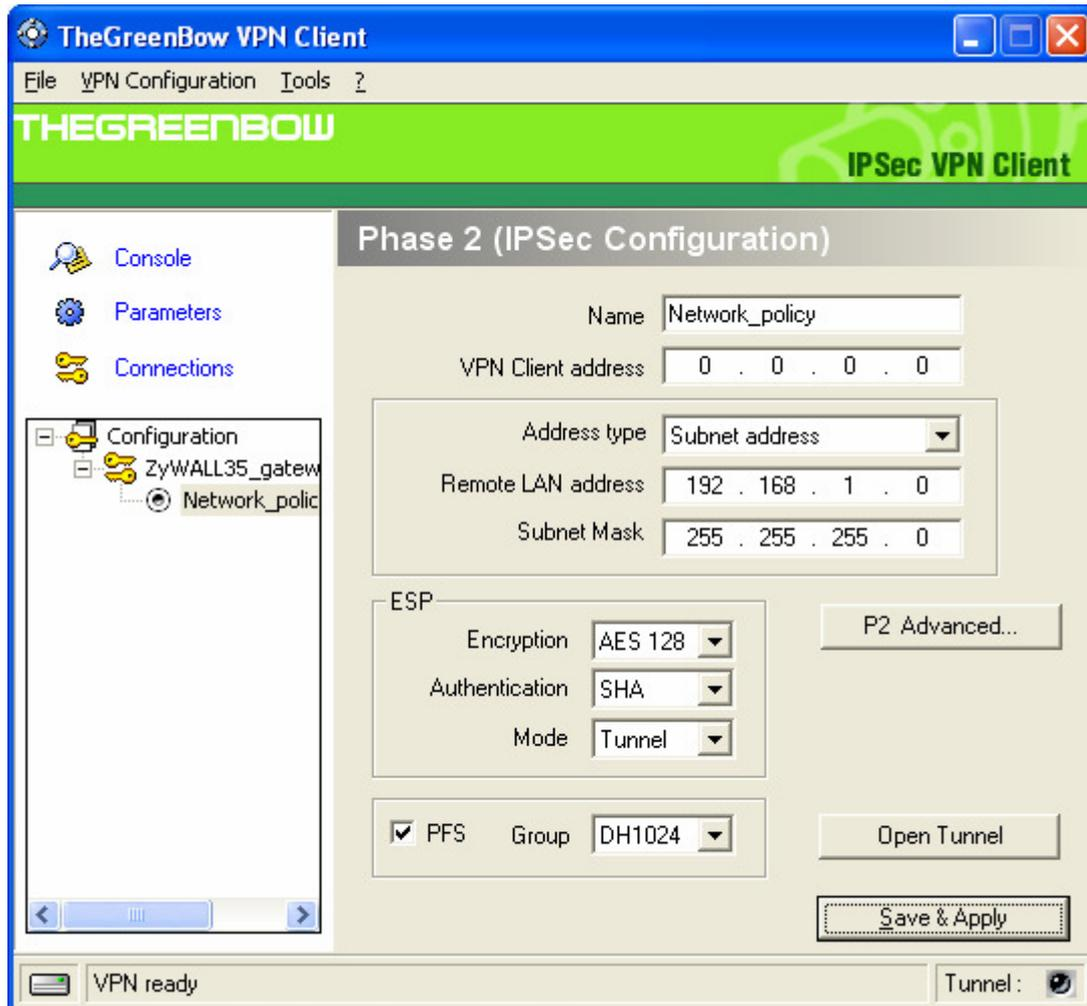
Modify Address type by choosing subnet address, and add the remote lan address and mask (must match what was defined on ZyWALL)
