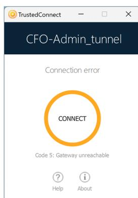
An orange connection status indicator ring, an error code, and a brief message describing the error are shown in the TrustedConnect panel to identify the main error cases.
